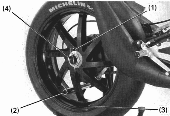
(1) LOCK PIN (2) STOPPER (3) REAR WHEEL (4) WHEEL NUT (LEFT-HAND THREADS)
